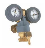
Mini pressure regulator with flow gauge, i.e. with indication I/min on secondary gauge. Integral safety valve. The flow is adjusted on the regulating screw by changing the secondary pressure and through a throttle valve in the outlet.
